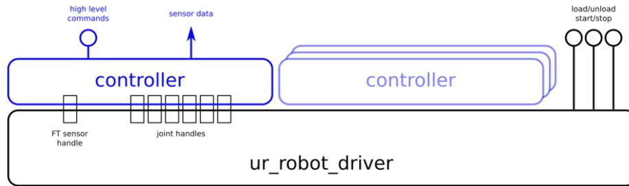
Figure 4 - A ros\_control based driver with a single active controller (dark blue) and multiple stopped controllers (light blue). Controllers can be switched in real time using ROS services.
