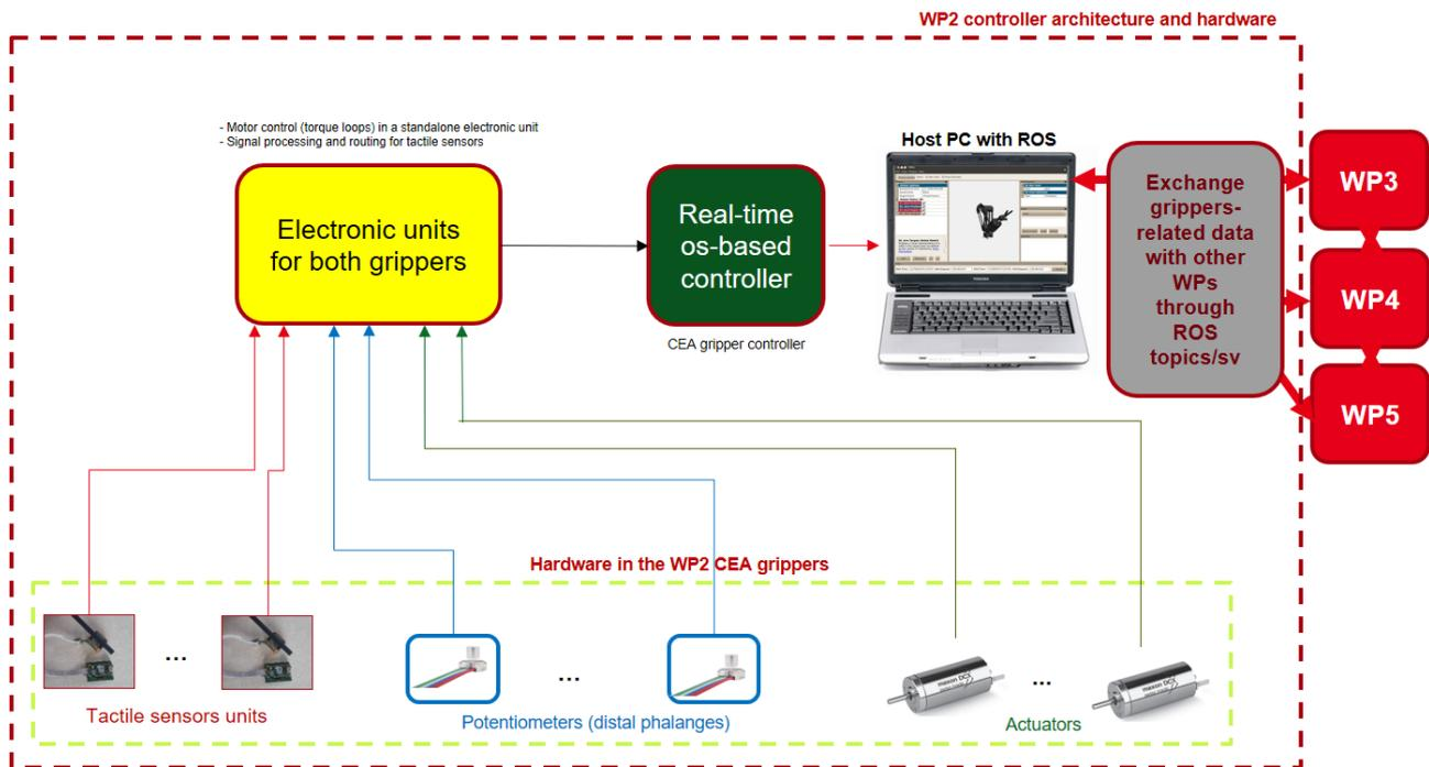
Figure 11 - Hardware and software interfaces between CEA gripper developed in WP2 with respect to other WPs.
