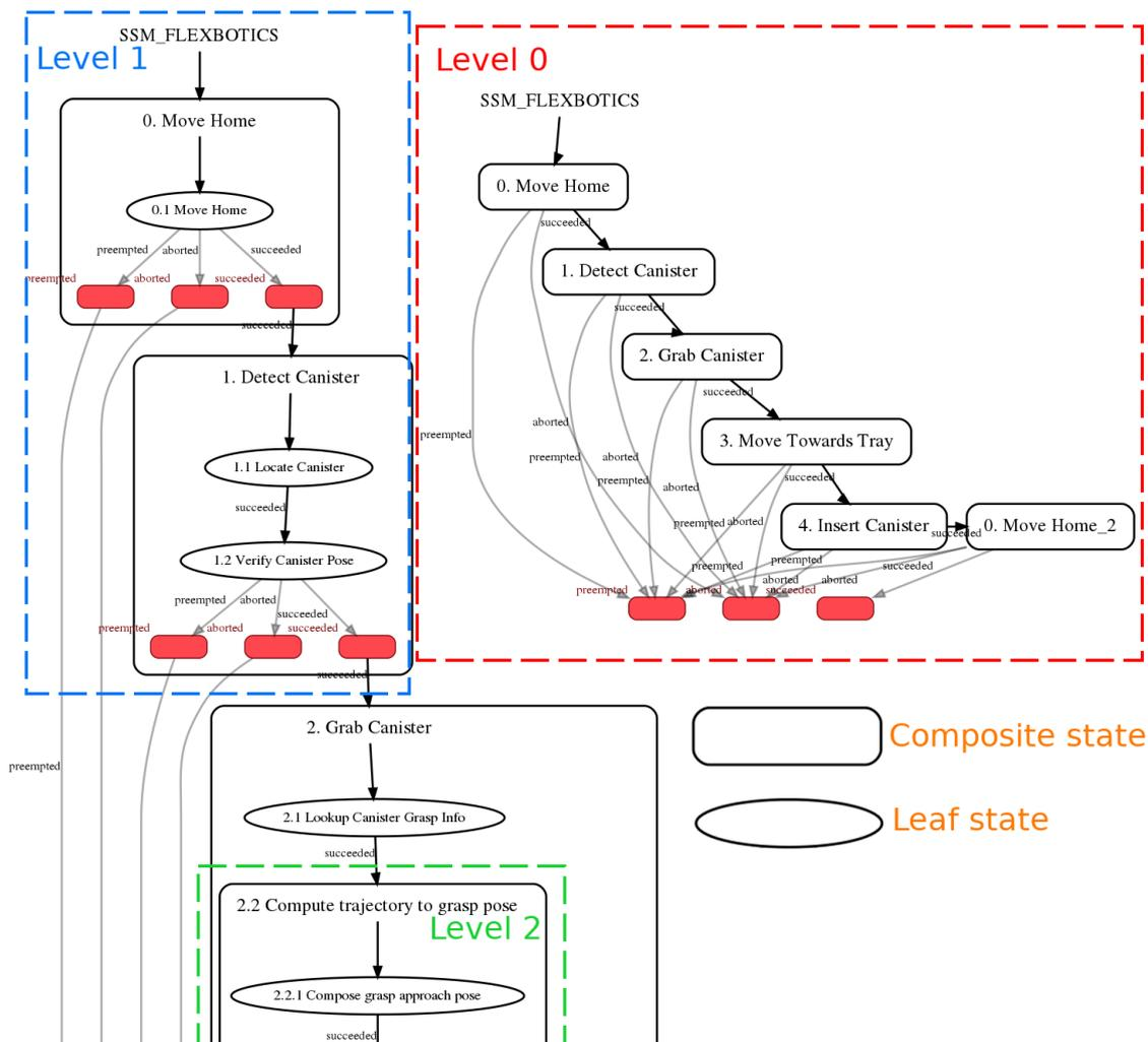
Figure 3 - Hierarchical finite state machine generated by the Skill Execution Engine. Based on the sequences of behaviours described in the simplified use case process file, *insert canister*.
