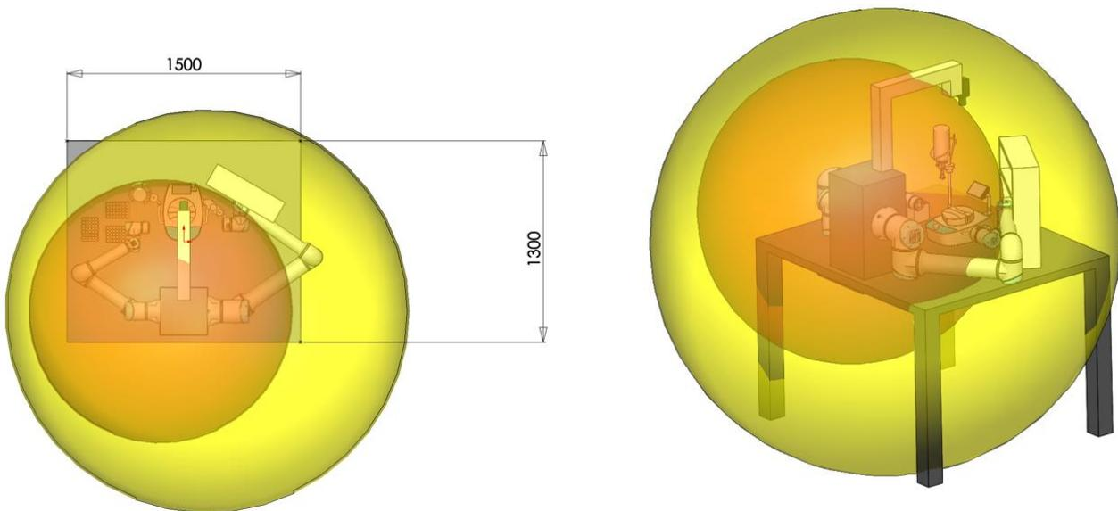
Figure 9 - Reach comparison between UR5e Robot Arm (Red Sphere) and UR10e Robot Arm (Yellow Sphere)
