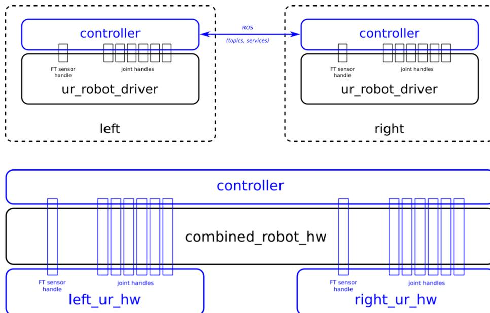
Figure 5 - A system with standalone drivers coordinating using ROS primitives (top) is much less efficient than a composite driver where a single component can directly access resources from both robots (bottom).
