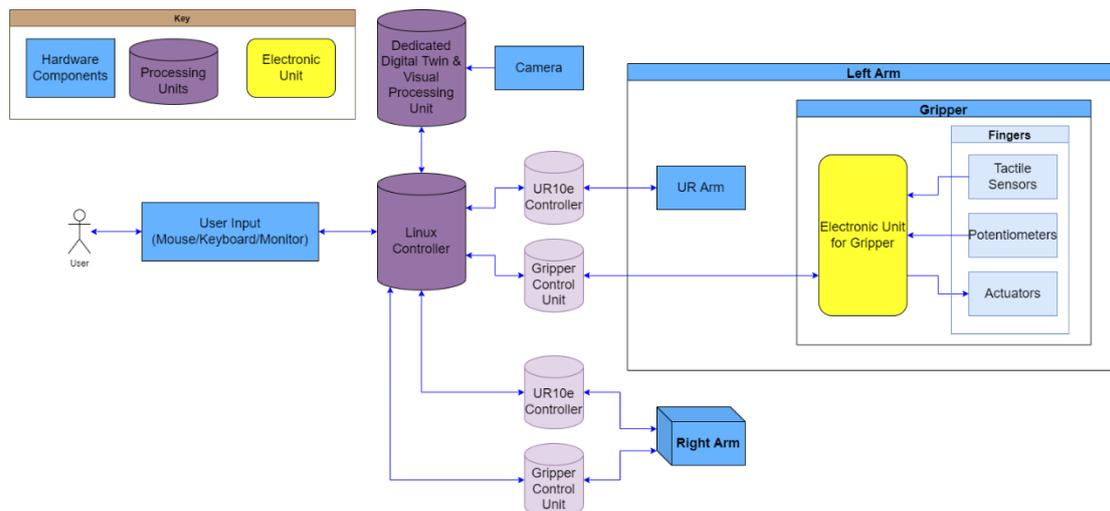
Figure 6 - Hardware Framework Flow Diagram
