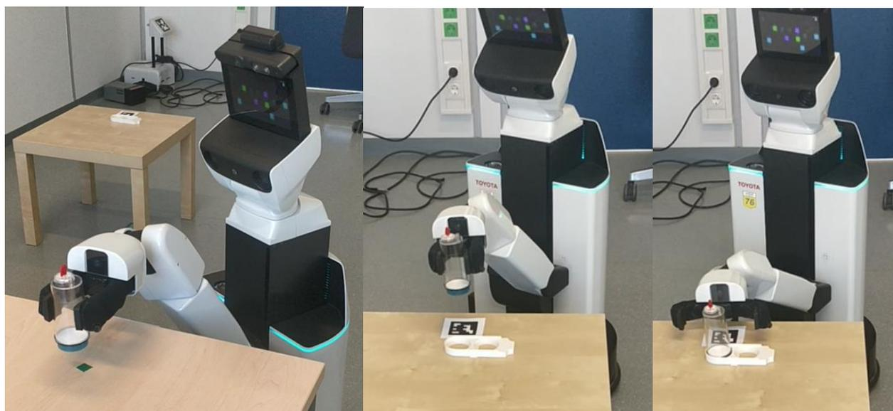
*Fig. 15: Example manipulation using visual detection of the canister and the tray. Performed with the Toyota HSR robot at TU Wien.*
