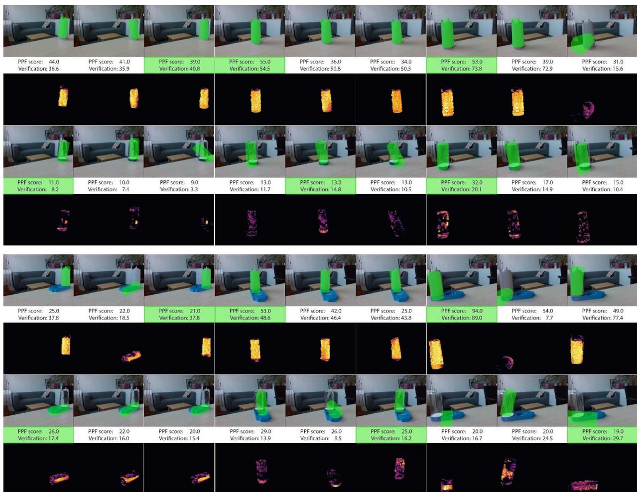
Fig. 14: The top-3 PPF hypotheses for three different views (left to right) and the corresponding per-pixel verification score (brighter color indicates better alignment). We compare results for (top to bottom) the spray-painted canister and the original transparent canister in isolation as well as both versions in the tray.
