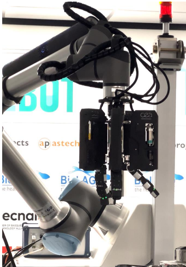
Figure 6 : External Hardware Components of the CEA Gripper
